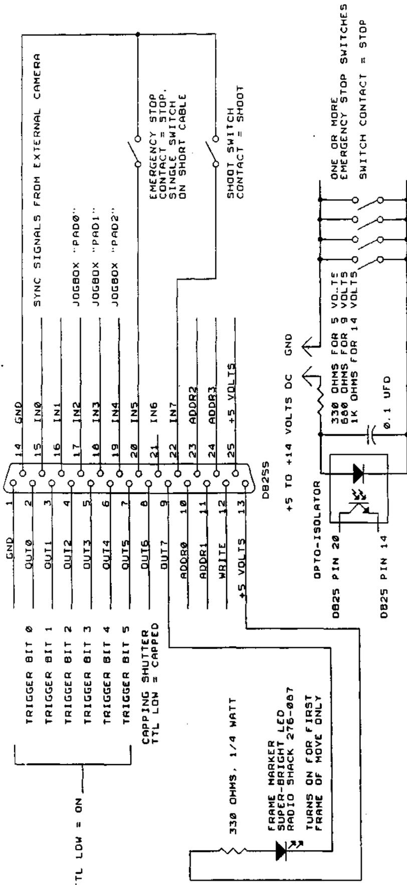
USE THIS SCHEME IF YOU WANT TO USE SEVERAL EMERGENCY STOP SWITCHES. ALMOST ANY OPTO ISOLATOR WILL DO, ALTHOUGH DARLINGTON TYPES MAY BE TOO NOISE SENSITIVE. \*\*DO NOT USE THE COMPUTER POWER SUPPLY TO POWER THIS CIRCUIT!\*\*
