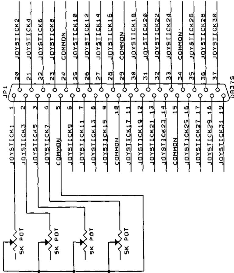
THIS PINOUT APPLIES WHEN THE 40 PIN JOYSTICK HEADER "JPI" IS BROUGHT OUT TO A DB37 CONNECTOR IN THE IBM I/O SLOT AT THE BACK OF THE COMPUTER. THE DRAWING SHOWS THE APPEARANCE OF THE CONNECTOR IS AS VIEWED FROM THE BACK OF THE COMPUTER.
